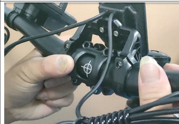
05.Fit the stem and handlebar together
