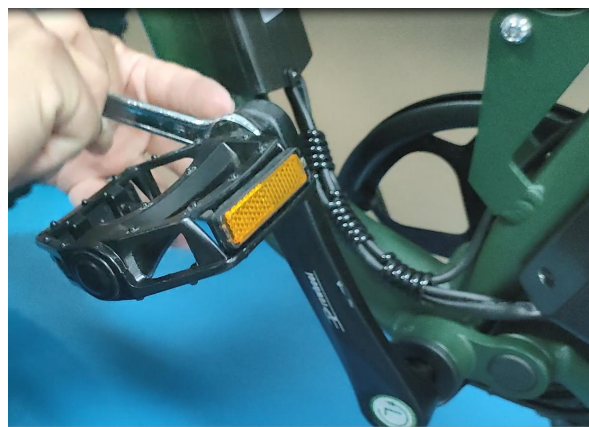
23. Tighten the pedals by wrench. Please note the direction of rotation
