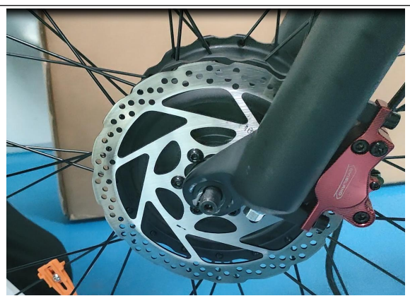
06.Put the disc rotor into the caliper and put the axle into the hook on the bottom of the fork. The protruding washer is inside the fork
