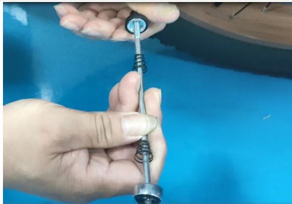
11.Unscrew the nut of the skewer, remove one spring
