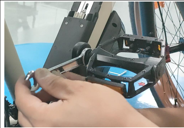
25. Tighten the pedals by wrench. Please note the direction of rotation
