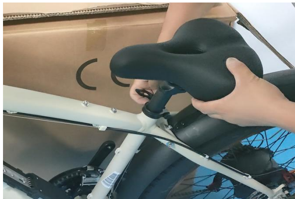
23.Insert the seat post, tighten the nut and quick-released lever
