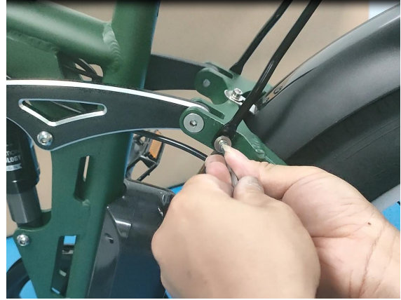
26. Then tighten the top bolts
