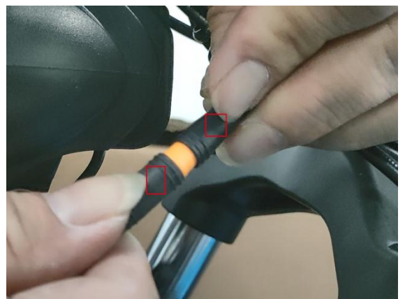
22.Connect the headlight cable (align the arrows)
