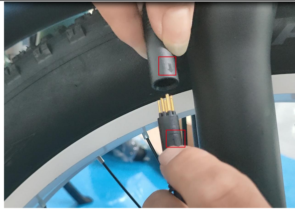
19. Align the arrow of the front motor cable and connect it
