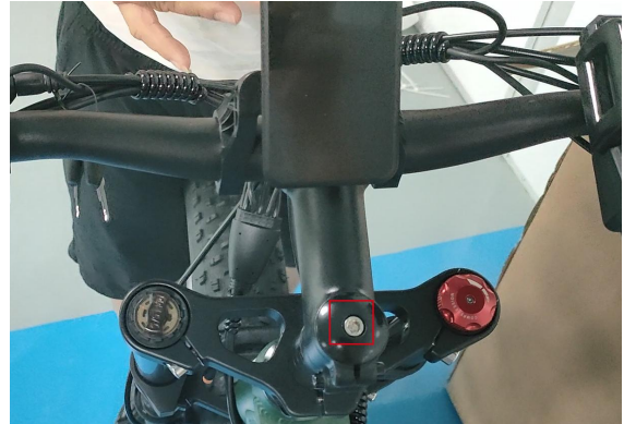
12.Tighten the top bolt
