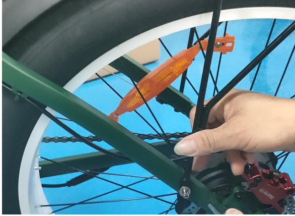
25. Tighten the lower bolts first
