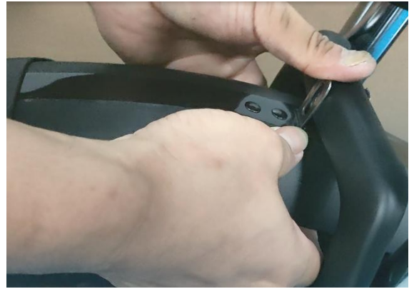
20.Install the front fender (the two iron plates of fender clamp the arch of fork)
