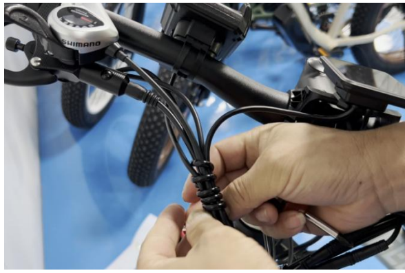
19.Sort the wire harness, put the phone holder cable inside the harness
