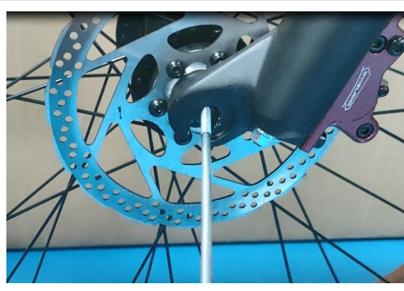
12.Insert the skewer from the disc brake side
