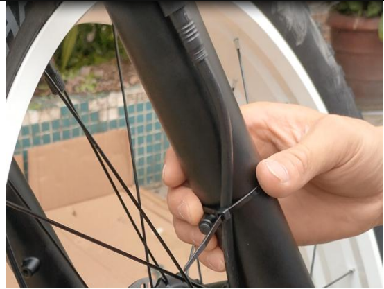
20. Secure the motor cable to the fork with a cable tie. The motor cable should be kept away from the tire to prevent friction
