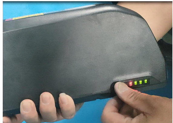
30. Then press the battery indicator light button, there will be 4 lights on; release the button, lights off
