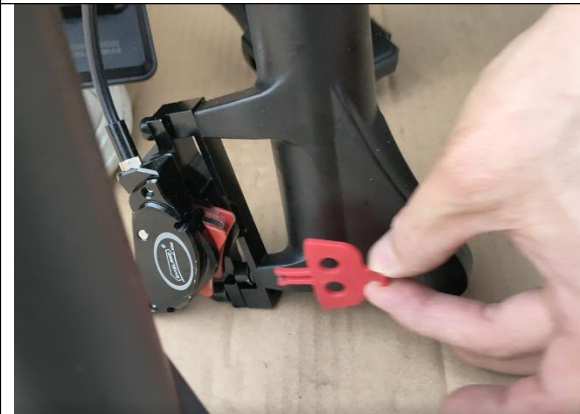
03.Remove the spacer in the caliper on the fork
