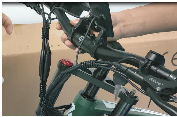
09.Fit the stem and handlebar together
