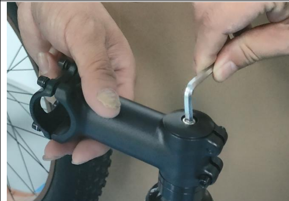
03.Tighten the top bolt
