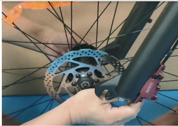
09.Put the disc rotor into the caliper and put the axle into the hook on the bottom of the fork
