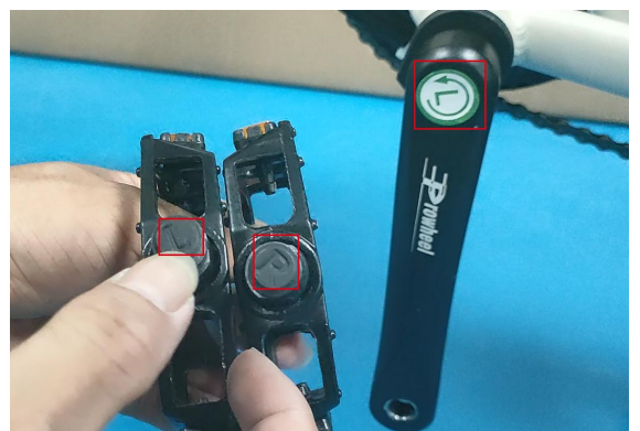
24.Put the Left & Right pedals correctly into the cranks
