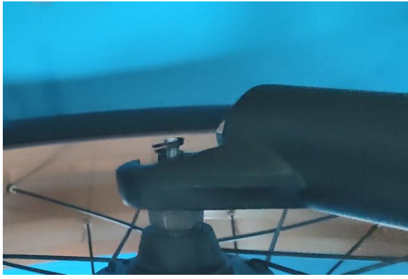
13. On the other side, put the spring (the larger side of spring faces outward)
