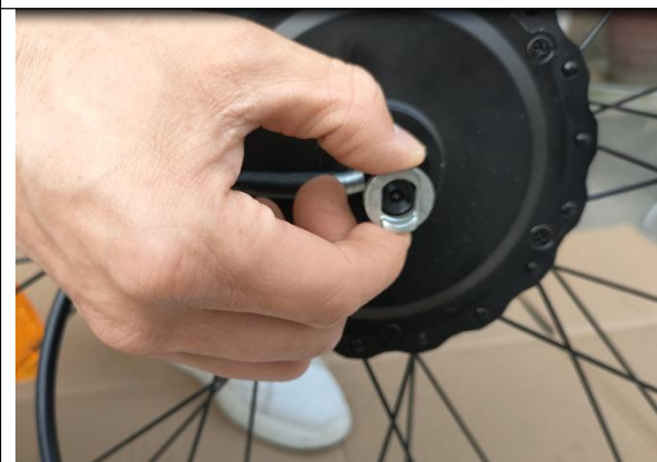
05.The motor wire should be on the right side, and backwards. Put this protruding washer on both sides of the motor axle, the protruding side should face outward and downward
