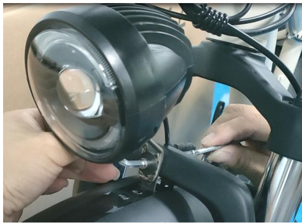
21.Install the headlight, tighten the nut by wrench
