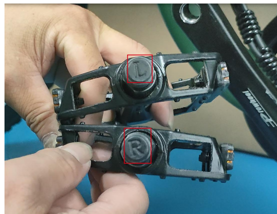
22. Put the Left & Right pedals correctly into the cranks
