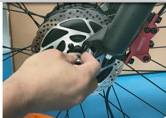
04.Remove the nut and protruding washer on both sides of front motor axle
