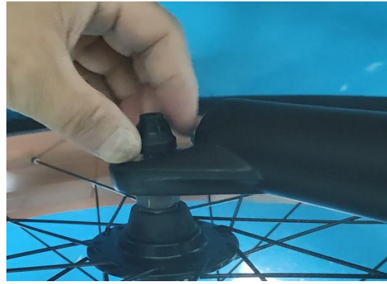
14. Tighten the nut of skewer until the lever becomes firm to close
