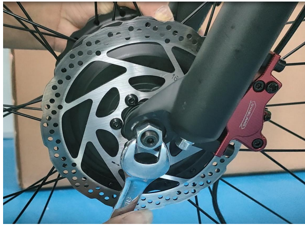
07.Put the nut and tighten them on both sides by wrench
