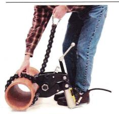
Using hand ring, pull chain over pipe and under tie bolt, then up between jaws as tightly as possible.
