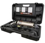
The Kinetic Water Ram uses a burst of compressed air that drives a shock wave (kinetic energy) through water to break up the blockage. Great for when the blockage is on the far side of tight bends, since the shock wave travels through water around bends without losing force and is not affected by stacks or vents. Instant impact with no build-up of pressure in the plumbing system.
