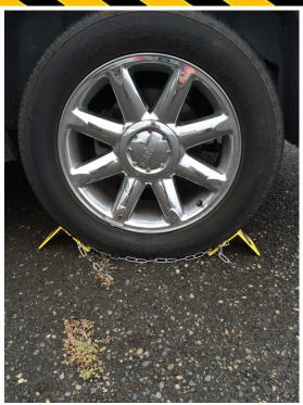
Step 1: Place a wheel chock in front of and behind a wheel.
