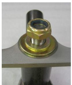
The center photo shows the placement of the optional shim. The shim is OPTIONAL. It is simply used to fill small gaps caused by wear or part variation between different manufacturers. As the bushing in the mounting socket wears down in height, you may add a shim washer if you like. Unless bushing wear is severe, the shim washers are for aesthetics only and do not affect normal operation.
