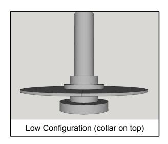
This tool will accommodate travel down to within about one inch of the base. However, at the low end of the tool's travel, the hardware heads from the plate and base mounting may interfere with travel. If you need more downward travel than you are getting, you can try to offset the hardware or get in touch with us for countersunk hardware.
