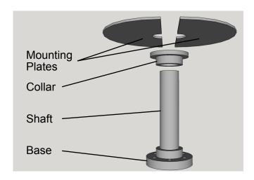
To use this tool, insert the shaft into the base, and run the threaded piece through the center of the assembly from the bottom, seating the base of the threaded piece into the slot in the tool base. Use the included hardware to put a nut on the top and tighten the assembly. Then bolt the tool base to the crankshaft hub, normally with your flywheel/starter ring in place.
