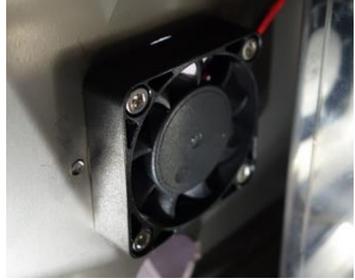
Figure 41: Shows 4 x M3 socket screws securing fan
