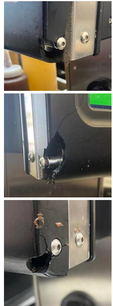
Figure 34: Examples of over-tightening (extreme cases)
