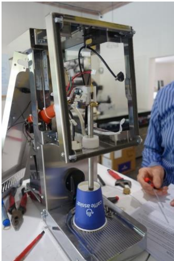
Figure 28: Ideal servicing height. Use an upturned cup for easy access of the wand carrier assembly
