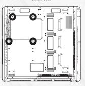
Attach the stand-offs according to your motherboard form factor. Attach the included EPS extension cable on to your motherboard – do not connect it to the power supply yet.
