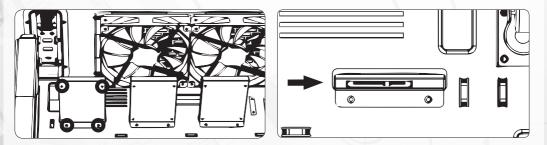
3. Removing the front panel and top cover
