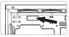
Fix the motherboard to the motherboard tray. After the installation of the power supply, you can connect the EPS extension cable to the EPS-connector on the PSU at the underside of the motherboard-tray.
