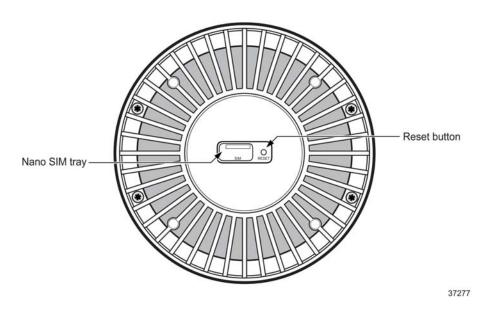
The SIM card slot is for a 4FF/nano-size SIM card on the bottom of the device.
