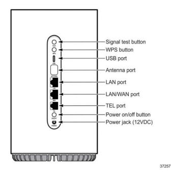
Two RJ-45 LAN ports can be used for the following:
