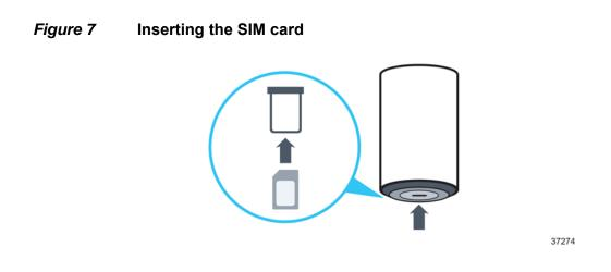
Remove the SIM tray using the finger grove. Place the SIM card in the tray and insert it back into the gateway.
