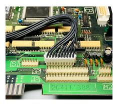
12. For optional spinner switch only; connect the other end of the 3-pin switch harness to JP3 with the exposed contacts facing towards the JAMMA edge. There is no harm in plugging the harness in backwards, it will just reverse the operation of the joystick/spinner switch.
