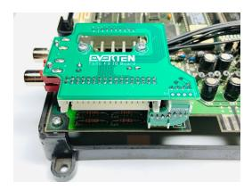
10. For Lions3 case only; as the board lowers into position ensure the stereo PCB is positioned underneath the custom Lions3 left riser screw tabs.
