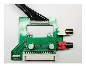
8. For optional spinner switch only; connect the 3-pin switch harness to the JP3 connector on the stereo PCB.
