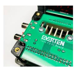
11. Connect the other end of the 10-pin kick harness to the AA connector on the Taito F3 PCB.
