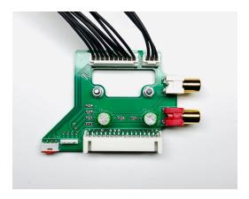
9. Slowly screw the stereo PCB into the heat sink, alternating screws every couple of turns. As you lower the board into position ensure the S headers are aligning and inserting into the interconnect board socket.
