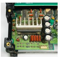
5. Remove the protective cap on the S connector of the stereo PCB.
