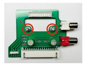
7. Connect the provided 10-pin kick harness to the AA connector on the stereo PCB.
