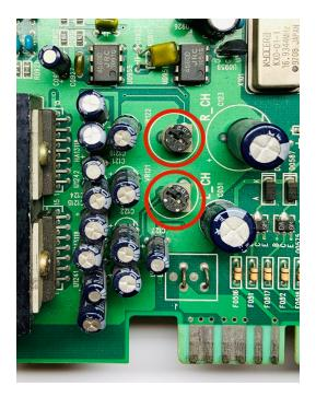
3. Screw the thread-forming screws (colored heads) into the 2 holes on the audio heat sink. These screws will create threads for installation of the brass standoffs. Go slow and **DO NOT** overtighten or you will strip the threads you've created.
