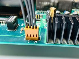
7. Mount the stereo PCB to the brass standoffs using the 2 x 6mm mounting screws. Ensure the screws firmly holding the board down. These screws provide a necessary ground connection between the stereo PCB and the Seibu SPI PCB.
