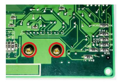
5. Align the bottom stereo PCB board with the screw holes and check alignment of the castellated holes with the solder points indicated in Step 2. Using the screws you removed in the previous step, mount the bottom stereo PCB, using the brass standoffs included in the kit in place of the nuts.
