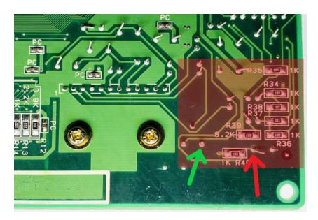
4. Remove the 2 screws from the audio amp shown in the picture below. Save the screws and washers, the nuts are not required for mounting the stereo PCB.
