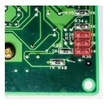
2. Ensure the pads of R36, R37, and R38 are clean and flat. Adding some fresh solder to both sides of R35 will making installation easier as well. You will be soldering the bottom stereo PCB to these connections for routing to the top stereo PCB in a later step.
