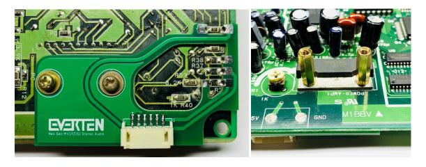
6. Carefully solder the 6 castellated holes on the bottom stereo PCB to their respective connections on the MVS board.
