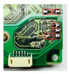
7. **IMPORTANT!** Verify continuity with a multimeter from test points in the diagram below back to the bottom stereo PCB wire harness connector legs. On some MVS boards, test points 1 and 2 may have solder mask preventing good continuity readings. Alternate test points can be found on the reverse side of the board on OPAMP1. Test point 1 = OPAMP1 pin 8, Test point 2 = OPAMP1 pin 14.
