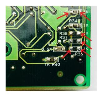
3. If possible, straighten any bent through-hole component legs in the highlighted area in the picture below that could interfere with installation. An example of a bent leg indicated by red arrow; straight leg indicated by green arrow.
