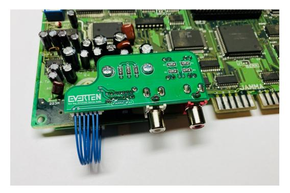
9. Move the sliding switch to the right position for stereo RCA or to the left for JAMMA mono. **Do not adjust the switch while the MVS is powered on.**
