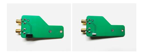
5. Attach the 19mm nylon standoff to the stereo PCB using the provided 6mm screw.
