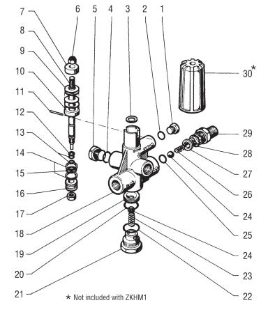
Note: For proper operation of the HM Unloader, it must be mounted in the vertical position. The optional spring (item #23) must be used if the unloader is mounted in any position other than vertical.
