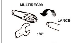
Fit the MULTIREG99 on lance tip with 1/4" threads. Use Teflon tape or an anaerobic thread sealant to reduce the risk of leakage. Tighten using a wrench only on the brass flats on the inlet fitting of the Multireg.
