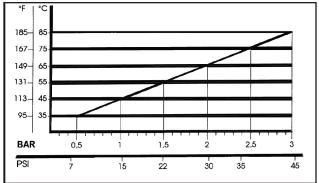
Naturally, if the application allows for feeding the pump with 45 psi (3 bar) even at low temperatures (for example: 1150F/450C the life of the wet end of the pump will be even longer.
