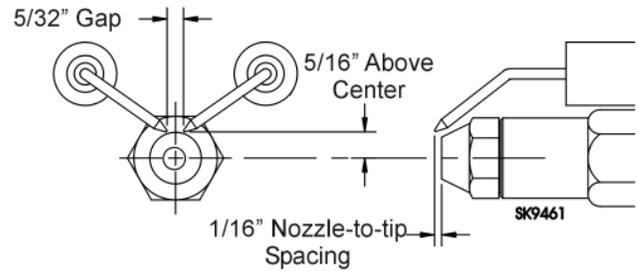
The Dimensions shown below are for use with L2 heads and M series air tube combinations ending with an 'N' suffix (example: AFG70MDAQN)
