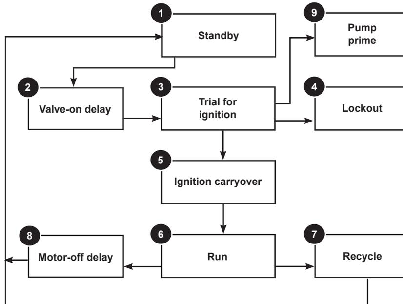
1. **Standby:** The burner is idle, waiting for a call for heat.
