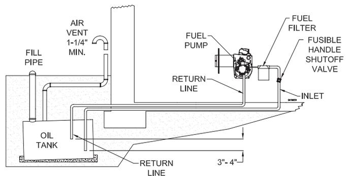
**NOTICE** To further protect the fuel supply system and reduce nozzle orifice plugging with firing rates below 0.75 gph, a dual filtration system can be installed. This typically consists of a 50 micron primary filter, located near the fuel tank and a secondary filter rated for at least 10 microns located near the burner.
