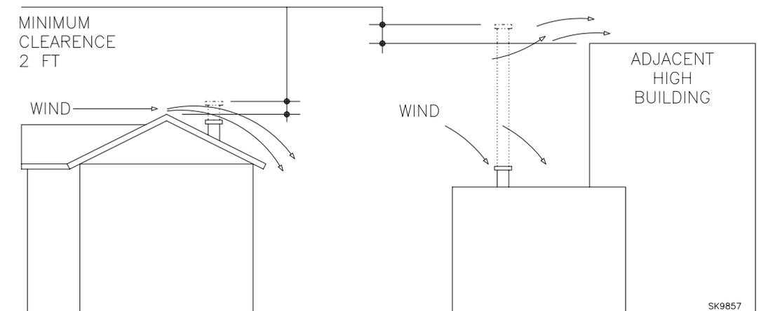
**NOTE:** Correct chimney design is shown by dotted lines. Incorrect chimney design, as shown by the solid lines, may result in down-drafts.
