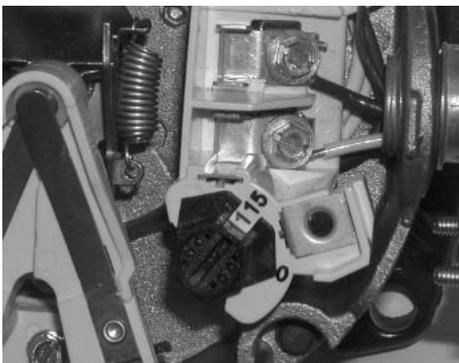
**Figure 13 - Motor Set for 115 Volt Operation**
