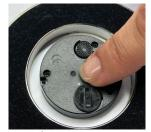
Turn battery compartment cover counterclockwise, using fingernail or screwdriver.
