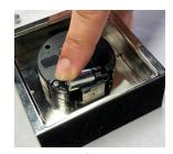
Insert "N" battery. Follow+ and - polarity. Return assembly to case. Replace center knob, turning clockwise to tighten.
