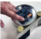
Insert "AA" battery. Follow + and polarity. Replace back plate and turn knob clockwise to
