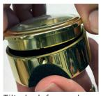
Tilt clock forward and remove mechanism assembly from base.
