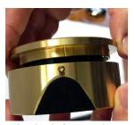
Tilt clock forward and remove dial/mechanism assembly from case.
