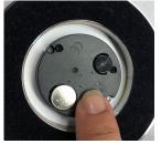
Insert button cell battery. Follow + and - polarity. Replace cover and turn clockwise to lock.
