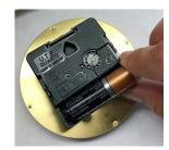
Insert "AA" battery. Follow+ and - polarity. Return assembly to base, aligning top notch. Replace bezel, turning clockwise.
