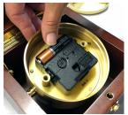
Insert "AA" battery. Follow+ and polarity. Replace back plate and fasten knobs.
