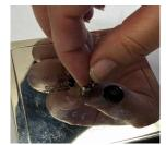
Unscrew center knob on back of clock. Turn counterclockwise.
