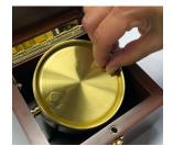
Unscrew both brass knobs on clock back plate.
