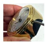
Turn base screw counterclockwise one turn. Do not remove screw completely.
