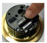
Insert "N"battery. Follow+ and polarity. Return assembly to base, aligning notch. Tighten screw, turning clockwise.
