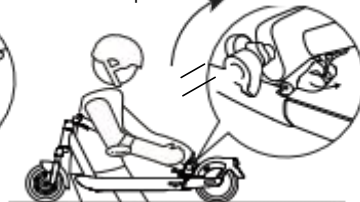
Press down the folding ring and lift up the mast
