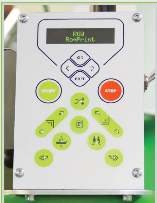
:: PIEZO CONTROL PANEL: MOVEMENT AND POSITIONING OF THE SCREEN; RECORDING AND MEMORIZATION OF THE SCREEN POSITION
