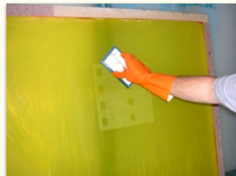
2. Scrub screen with non-abrasive pad or brush. Allow product on to dwell on screen 2 to 5 minutes.
