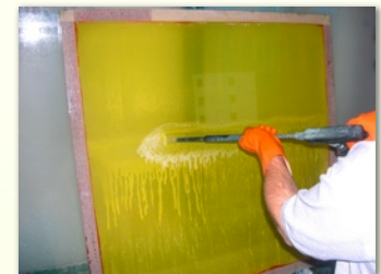
3. High pressure rinse - starting at bottom on the print side of the screen. Reverse screen and high pressure rinse.
