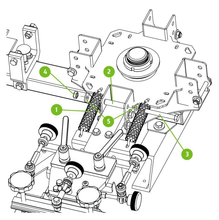
Mount the press base feet (2) to a sturdy tabletop with supplied mounting screws (1). Press is shown mounted on a Riley Hopkins 1-station press cart (sold separately). A Phillips screwdriver is required for this step.
