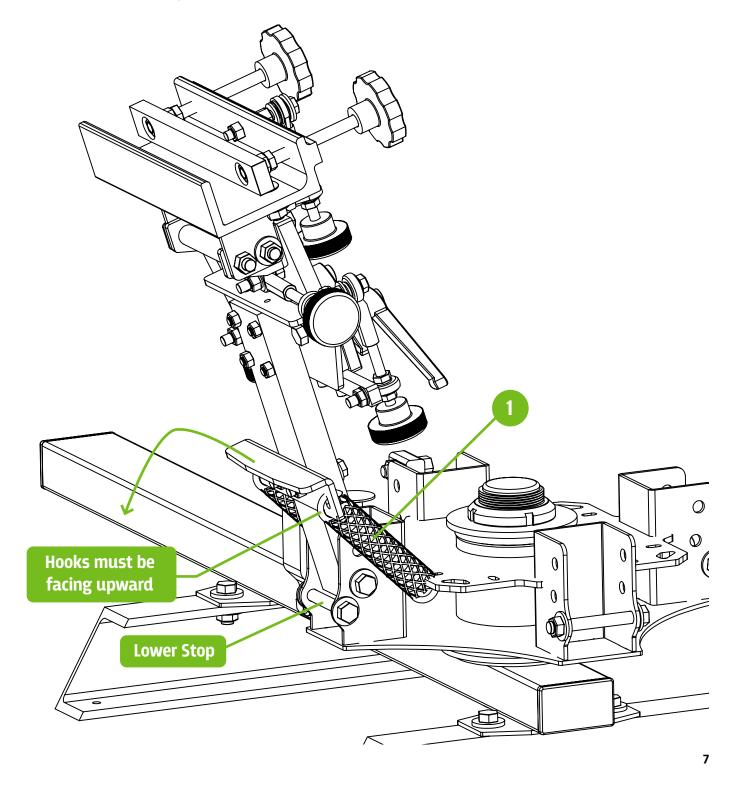
Install the upper stop bolts and rubber sleeves. Two 9/16" wrenches are required for this step. **DO NOT OVERTIGHTEN THE BOLTS**. This will cause resistance in the print head hinge point. Repeat this step for the remaining print head assemblies.
