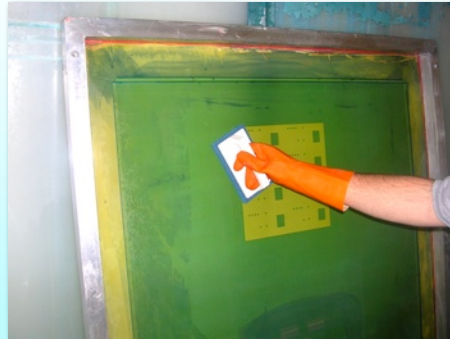
2. Scrub screen with non-abrasive pad or brush. Allow to dwell for 1-3 minutes.
