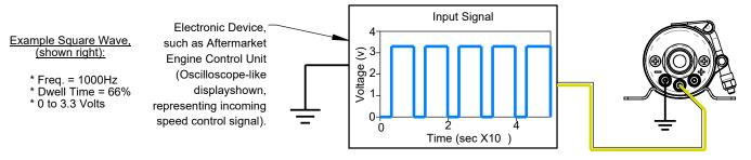
Refer to above Example 5, for use with the Fuelab Electronic Fuel Pressure Regulator, Models 52901 and 52902, that creates its own pulsed signal. These regulators automatically control the fuel pump, without the use of switching means or other components such as described in examples 2 and 3. Refer to instructions for the Electronic Regulator for proper wiring and installation.
