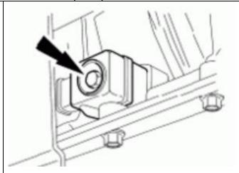
10. Disconnect the output shaft speed (OSS) sensor.
