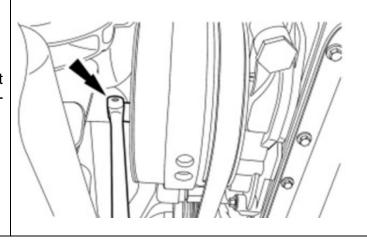
19. Remove and discard the 8 torque converter-to-flexplate nuts.
