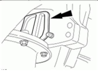
17. Remove the steering dampener-to-frame bolt and nut and position the steering dampener aside.
