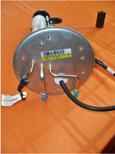
(Fig. 1) PS-123 Sending Unit mounting plate, showing bolt holes to be plugged.
