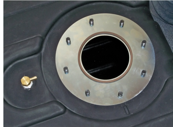
(Fig. 10) Center adaption “O” ring on top of adaption flange.
