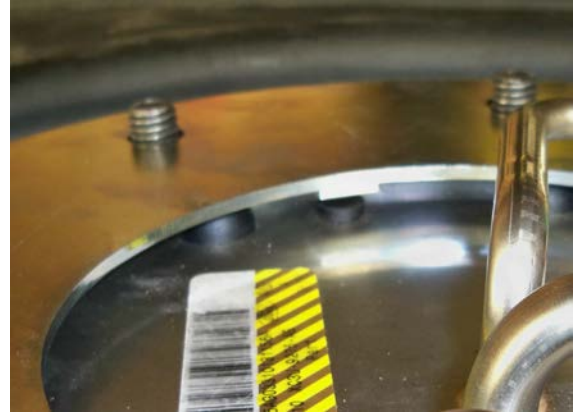
(Fig. 6b) Align tabs with small rubber plugs.
