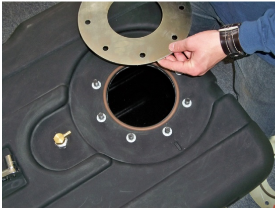
(Fig.9) Place one adaption flange on top of the tank's sealing “O” ring.
