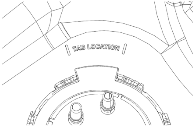
(Fig. 3) Line sending unit tab up with "TAB LOCATION" marks on tank.
