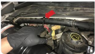
Double check to make sure the grommets are still on the truck after removing the stock intake box.
