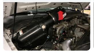
Disengage the red locking clip, press down on the tab, then pull out to disconnect the MAF sensor harness from the MAF sensor. Disconnect the filter minder electrical harness.
