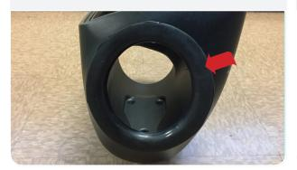
Garefully remove the MAF sensor from the stock intake tube then install the sensor onto the Intake Tube (C) with the 8-32 Screws (M), MAF Plate (H) and MAF Gasket (G). Install the Filter Minder Grommet (J) into the intake tube.
