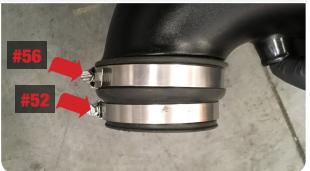
Install the Intake Tube (C) into the Air Box (A) then install the intake assembly into the truck. Align the fender side opening of the airbox with the inlet, then rock the airbox downward. Push down on the box to make sure that the air box is completely seated on the grommets then slide the coupler onto the turbo inlet.
