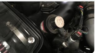
Reconnect the MAF sensor harness into the MAF sensor and engage the red locking clip. Reconnect the sensor harness into the filter minder.
