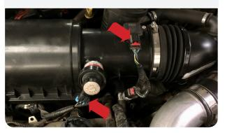
Disconnect the hose clip securing the secondary air inlet.
