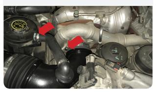
Lift the stock intake box to unseat the prongs from the grommets and remove both the intake assembly and secondary air inlet from the vehicle.
