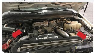
Loosen the hose clamp at the turbo inlet. Use a flat blade screwdriver to pry open the hose clamp securing the crankcase vent hose to the intake tube.
