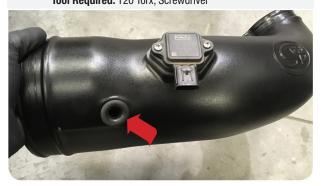
Determine if you want to install the Box Plug (S) onto the Air Box (A) or leave it open. See the "Air Box Plug" note on Page 2 for more information. If the Box Plug is desired, simply press the Box Plug into the box opening until it snaps into place.
