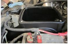
**11.** Spread the OE clamp open and remove the breather tube assembly from the OE intake tube.
