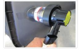
4 (B). If you have the OE "One Piece" intake tube, loosen the hose clamp at the turbo flange. Then Pull the OE breather tube from the valve cover.
