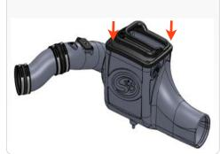
**29.** Reconnect the battery cables. Inspect your installation, make sure the kit is properly positioned and all fasteners are secure. Please keep your original air system and filter.
