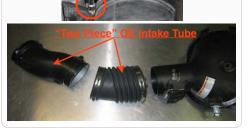
6. Remove the OE restriction gauge and gromm used later on during the install.
