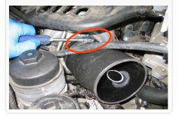
**Temp. Sensor NOTE:** If your vehicle uses a Temp. Sensor in place of a MAF Sensor: Use the supplied Temp. Sensor grommet (M) and install it in the hole of the intake tube (C). Once the grommet is installed insert the Temp Sensor into the grommet.
