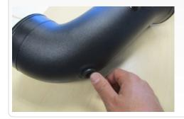
**19.** Place the Intake Tube (C) in the vehicle as shown, then rotate the tube so the MAF or Grommet is facing up.
