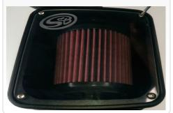
**28.** For increased airflow we recommend using the provided Inlet Lid, to seal off the box completely from foreign objects use the provided Clear Lid.
