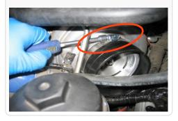
**12.** Install the large Grommet (T) into the Short Tube (P) followed by the 90 degree OE breather tube fitting.
