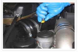
**26.** Reconnect the electrical connector to either the MAF sensor or Temp. Sensor located on top.
