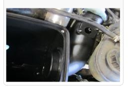
**23.** Secure both #72 Hose clamps after both tubes and coupler are aligned together straight.
