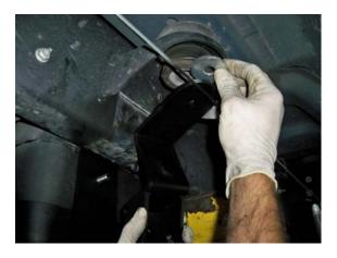
(Fig. 8) Place the supplied fender washer into the center of the rubber cab mount above the upper piece of the assembly.
