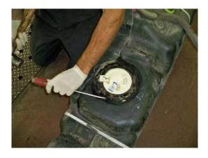
(Fig. 2) Loosen hold-down ring on original equipment tank by tapping counter-clockwise, remove and lift out sending unit.
