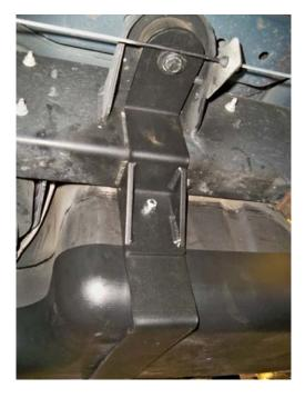
(Fig. 11) Completed front support installation on tank with TITAN Shield.
