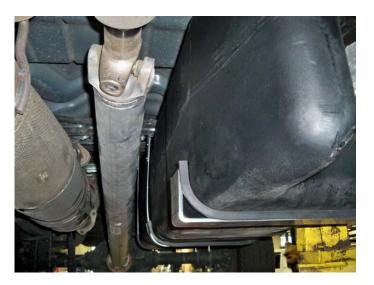
(Fig. 12) Installation of front support on tank without TITAN Shield. Note the flexible bushings on the support and the straps.
