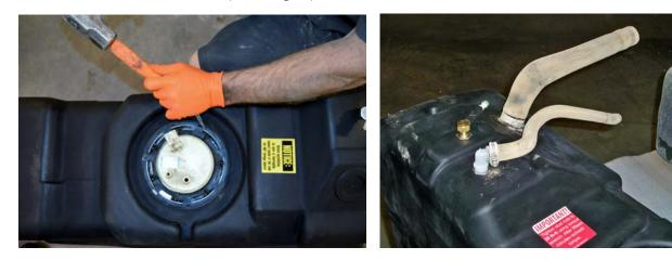
(Fig. 5) Using a hammer and punch, or screw driver to tighten the hold-down ring clockwise.
