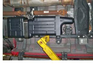
TITAN 2011+ Ford Crew Cab, Long Bed tank (7020311) installed showing three straps.
