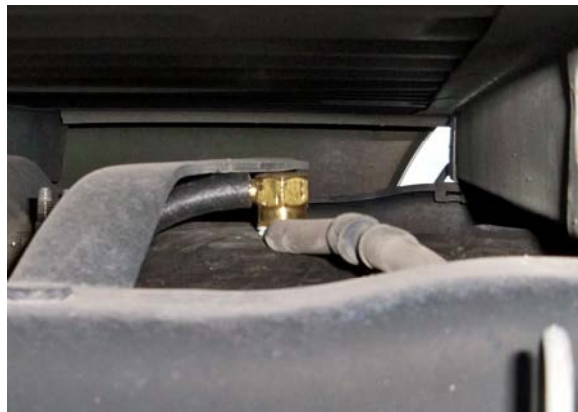
(Fig. 6) NOTE: Be sure that vent breather hose on rollover-stop vent valve, on the rear of the tank, is routed under the adjacent frame cross member as shown above.
