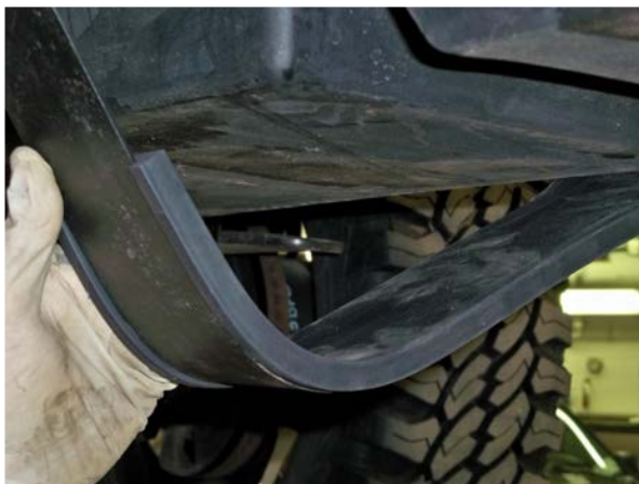
(Fig. 5) If optional TITAN Shield is not to be installed, install rubber bushings (pn 99 0000 0103) on both straps with the channel side toward the strap.
