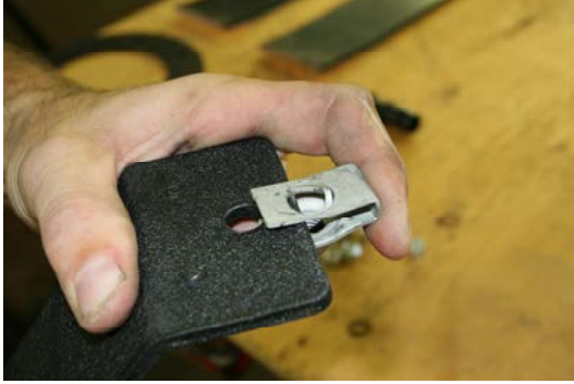
(Fig. 3) If vehicle has threaded clips, remove them from the OEM straps and place them on the TITAN straps.
