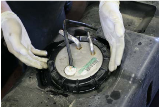
(Fig. 1) Loosen the hold-down ring on the OEM tank by turning counter-clockwise. Note where the connections on your vehicle’s sending unit are “clocked” and install so they are located in the same position in the new tank.
