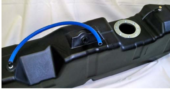
(Fig. 4) This photo shows the proper configuration of the \frac{3}{4} " vent line hose. When the tank is lifted into the vehicle trim it to proper length to attach to the fill spout vent. It must be configured to angle downward from the fill spout to the tank with no sags or kinks.
