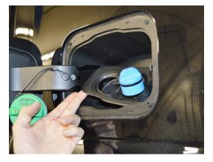
(Fig. 1) Loosen and remove rubber seal.
