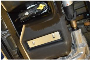
(Fig. 16) Tighten Front Support Assembly to 15 lb.-ft. (Fig. 17) Front Support Assembly properly installed.
