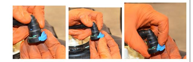
(Fig. 7): **Method for Disconnecting Fuel Line Couplings:** The majority of the couplings involved in this installation are of the quick connect type shown in left photo above. To disconnect, a) Slide the tab that has teeth on its edge outwards as shown in the center photo. b) Next, press the rounded button, as shown in the right photo, and pull the coupling apart. The coupling shown in Fig. 5 functions differently, see Step no. 9 for it.
