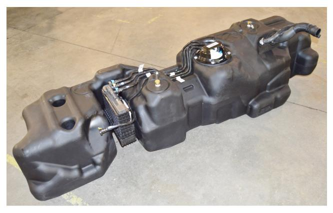
(Fig. 14) TITAN 7020217 tank shown with sending unit, water separator, fuel lines, sending unit guard, and fill and vent hoses installed; ready for installation into the vehicle.
