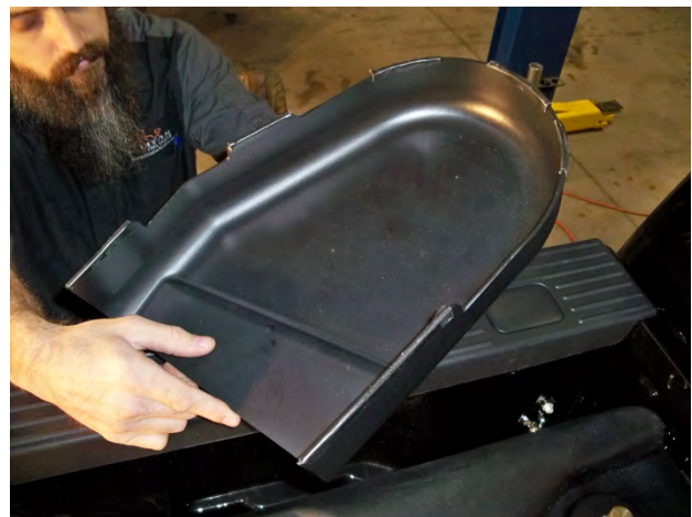
(Fig. 20) Place supplied double-stick tape in at least six Strips around bottom of Sending Unit Cover
