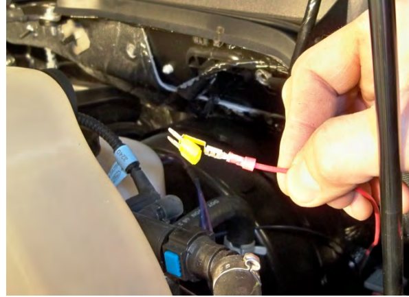
(Fig. 22) Using the supplied fuse tap, connect power input wire to output side of 10-15 Amp fuse (Max. 15 Amp).
