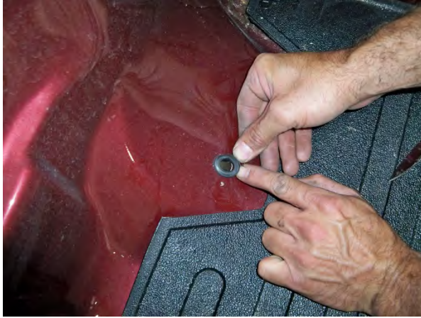
(Fig. 10) Install rubber grommet into transfer hose hole(s). (Fig.11) Assemble rear adjustable toe clamp assembly.
