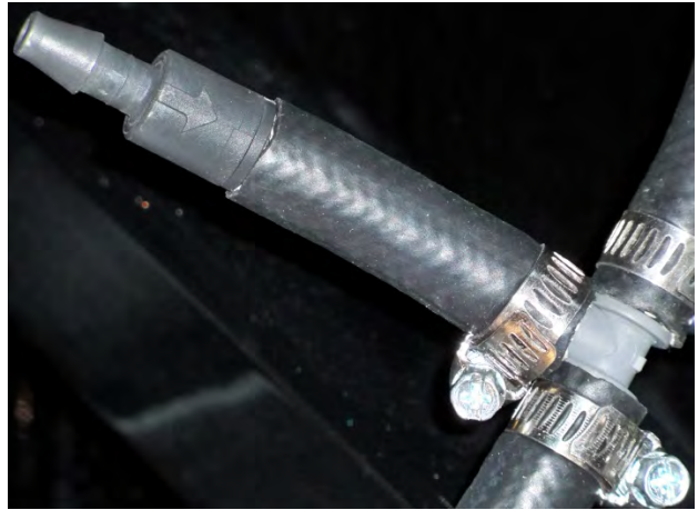
(Fig. 18) Shows 99 0000 0104 Check Valve Installed with directional arrow.
