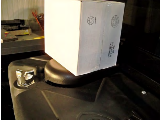
(Fig. 21) Place 20 lbs. of weight on Sending Unit Cover for at least 2 hours.
