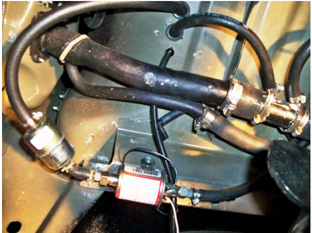
(Fig. 17) Transfer plumbing complete showing fuel filter in-line on suction side of pump. Notice fill hose adapter.
