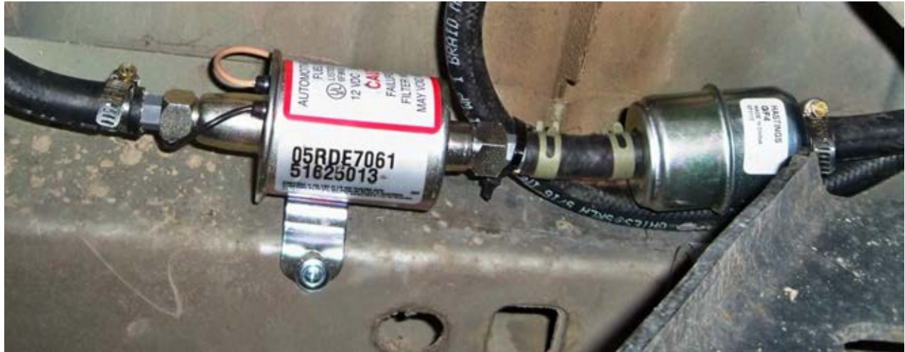
(Fig. 14) Fuel pump and inline filter installed.
