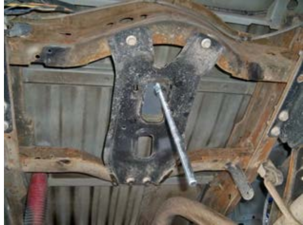
(Fig. 3) Cross member in 05-07 Ford vehicles showing STAFS top mounting plate & threaded rod installed.
