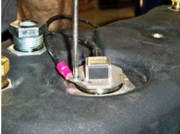
(Fig. 8) Connecting small eyelet end of grounding wire to top of electric fuel sensor. Other end attaches to chassis frame
