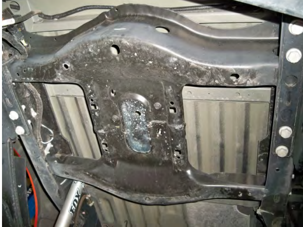
(Fig. 2) Cross member in 08-2014 Ford vehicles showing STAFS top mounting plate installed.
