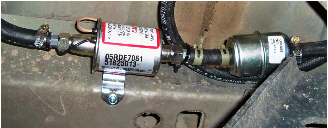
(Fig. 14) Fuel pump and inline filter installed.
