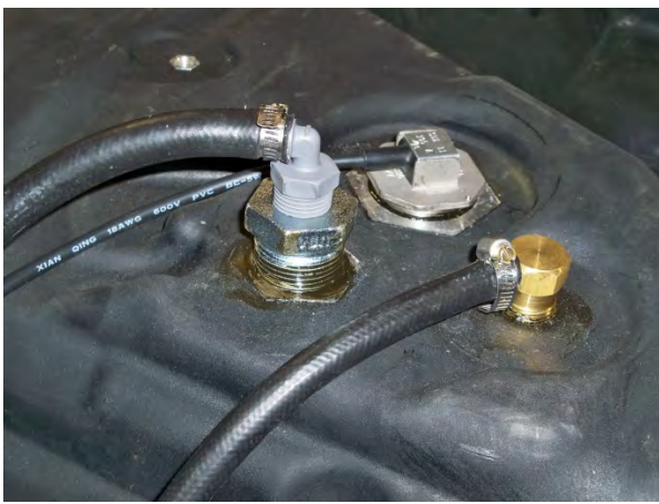
(Fig. 7) Install 5/16" hose onto the rollover valve as shown in this photo.
