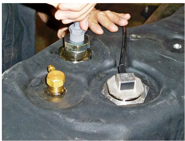
(Fig. 6) Installing 1/2" x 3/8" Hose Barb Elbow into plated Double Tapped Tank Bushing.
