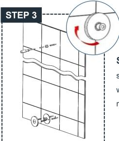
**STEP 3:** Insert one M4\*45 screw through the fixing block and two M4\*30 screws through the mounting seat and then secure them into the plastic wall anchors with an electric drill. Place the decorative cap onto the mounting seat and tighten it.
