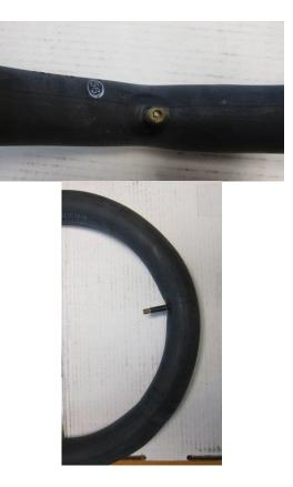
11. If there is a slow leak after a puncture, you must re-inflate the tire and continue to ride the scooter/e-bike some more. Most slow leaks will seal eventually once the latex has had a chance to cure. If a slow leak does not stop leaking, there could be a tear in the tube. Small tears (4-6 mm) will appear as slow leaks that never stop leaking air.
