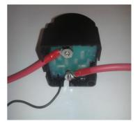
3. Using the red 110 amp cable you can measure, cut and make up your leads for the split charge circuit.
