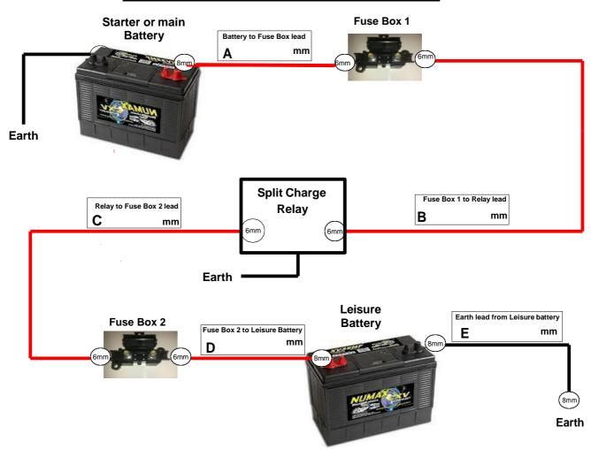
Before starting the instillation, the first thing you need to do is make a plan of where you're going to fit all your components and how long each cable will need to be. Have a look at the diagram above to see the basic wiring diagram of your voltage sensed split charge kit. I have left boxes on the diagram on the left to help you with your measurements.
