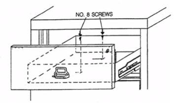
3. Each drawer has a drawer number decal on the right side and must be replaced in the same cavity it was removed from. The top drawer is #1. See the sketch below.
