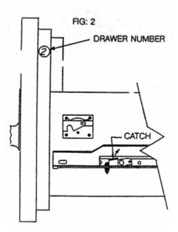
4. Place your index finger and thumb on the catch and release by pulling up on the drawer catch. See the sketch below
