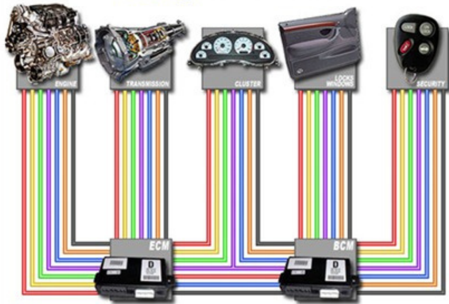
Vehicle Wiring: conventional multi-wire looms
