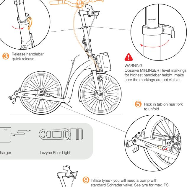
Perform a basic safety check before each ride as described in the User Manual. Check brakes are working. Check bolts, wheel nuts and quick release levers are tightened fully.
