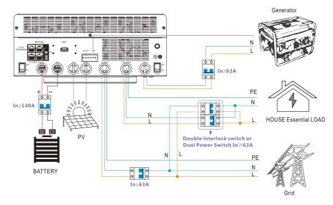
• The system will use AC first if there is both utility input and generator input.
