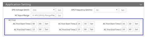
3.1 AC First: During this setting time, system will use AC to take load, use solar power to charge the battery first. If there is extra solar power, extra solar power will take the load. When out of the setting time, system will use solar and battery to take load first until the battery voltage/SOC is lower than On Grid EOD settings, then it will use AC to take the load.
