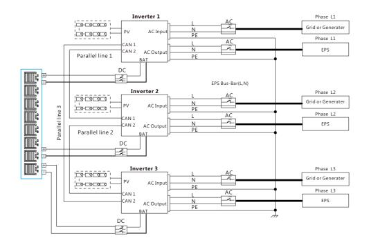
Step2. Please put the CAN communication PIN to on status for the first and the end inverter
