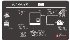
When display 'GRIDA', it means the Grid information is about AC utility, The percent display on the right down corner means the load percentage
