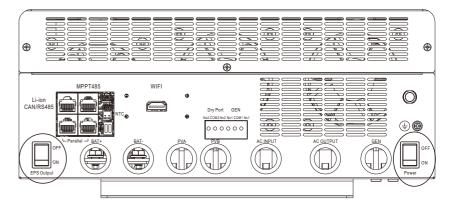
1. Power Switch: Control power supply for the unit
