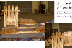
2. Insert pre-assembled table top into hole on each side of seat back (as shown). Next, repeat Step 1 for the remaining seat. Be sure that the table top is inserted into both seat backs before securing them to seat
