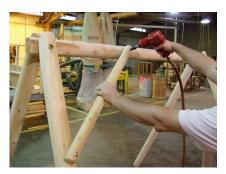
11. Stand frame upright and tighten 7 ½" machine bolts *only enough* to allow frame to stand freely. Measure 24" down from top of swing leg, and 24" in from end of top pole. At these points, use 4" lag bolts to secure the 24" braces to the swing (as shown in these two photos). Use ½" washers on each lag bolt. Now, tighten 7 ½" machine bolts firmly.
