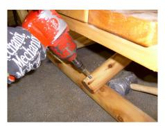
5. Use 3 3/8" lag bolt to secure angle brace to seat bottom. Use a 5/16" washer when inserting this lag bolt.
