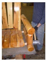
6. Attach both swing arm assemblies to swing seat. Align the two doweled ends of swing seat with the two holes in the swing arm assembly. Tap arms into place using rubber mallet or hammer. If using a hammer, be sure to pad impact area to avoid damage to the product.
