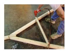
10. From machine bolt, measure 32" down swing leg. At this location, use 4" lag bolts to secure two of the 35" braces to swing legs. Use a 1/4" washer when inserting each lag bolt.
