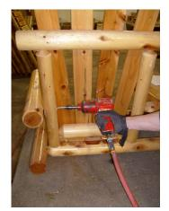
7. Find a comfortable angle for the seat back, use 3 3/8" lag bolts to secure the arms to the seat backs (as shown). Next, use 2" screws to secure all doweled insertion points. Use a 5/16" washer when inserting each of these lag bolts.
