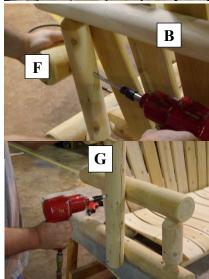
**Step 3:** Position seat back (**B**) at a comfortable angle and secure to the upper arm (**F**) with  $3\frac{1}{2}$ " lag bolt and 1/4" washer. Repeat process for opposite side.
