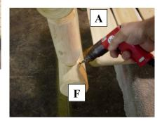
**Step 5:** Install 2" screw where all doweled ends are inserted, securing seat (**A**) (pictured) and seat back (**B**) to arm assemblies (**F**).
