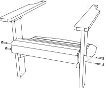
2. Attach (D) Back Assembly to (A) Seat Assembly (B) Armrest & (C) Armrest using 2- 2" Screws for Seat Assembly & 1- 1 3/4" Wafer Bolt for Armrest for each side. be sure to match all numbers and /or letters.tighten all Wafer Bolts with included Hex Key.
