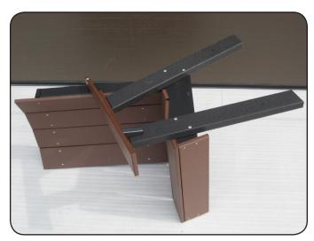
**Step 1**Using (2) 1/4" x 4" bolts back leg, (2) 1/4" x 3" bolts front leg, (1) 1/4" x 3 1/2" bolt arm, and (5) 1/4" nuts, attach legs (D) to seat (B) and back (A). DO NOT TIGHTEN NUT AT THIS POINT.
