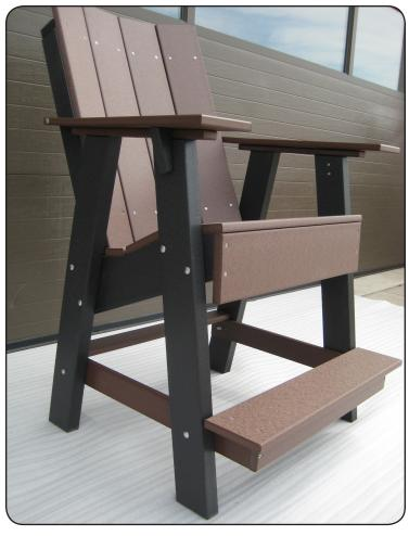
**Step 3**Using (4) 1/4" x 2 3/4" bolts and (4) 1/4" flange nuts attach the foot rest (E) to chair legs. Tighten using a 7/1`6" wrench or socket.
