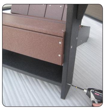
**Step 3**Now slide brace (D) in groove in front leg and fasten with (4) 2" screws.
