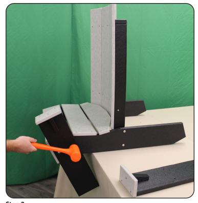
**Step 2**Using (2) 1/4" x 2 1/4" bolts and (2) 1/4" flange nuts attach legs (C) to seat, as shown. Repeat on other side.
