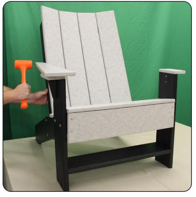
**Step 4**Attach the armrest (E) to the back with (1) 1/4" x 3 1/2" bolts and (1) 1/4" flange nuts. Repeat on other side.
