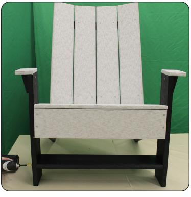
**Step 3**Now slide brace (D) in groove in front legs and fasten with (4) 2" screws, two on each end.
