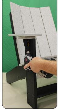
On the front of the armrest measure a 3/4" overhang on the inside as shown left, fasten the armrest using (4) 1 1/4" screws in the predrilled holes from the bottom up. Repeat on other side.
